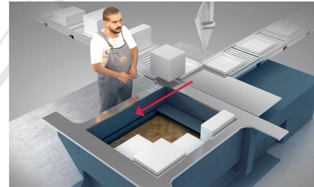
After staging the goods on the pallet, the full pallet is lowered automatically via the shaft to the shrink wrapping station. The shaft containment walls ensure that the load stays stable. This is especially important in pallets with mixed goods. As soon as the pallet is lowered, the shrink wrapping station contains the load automatically with a film. The goods are well-protected from slipping and ready for shipment.
